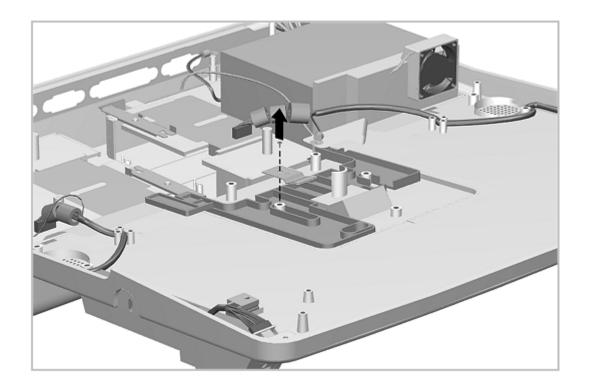
Figure 7-36. Removing the Puller Plate Spring
